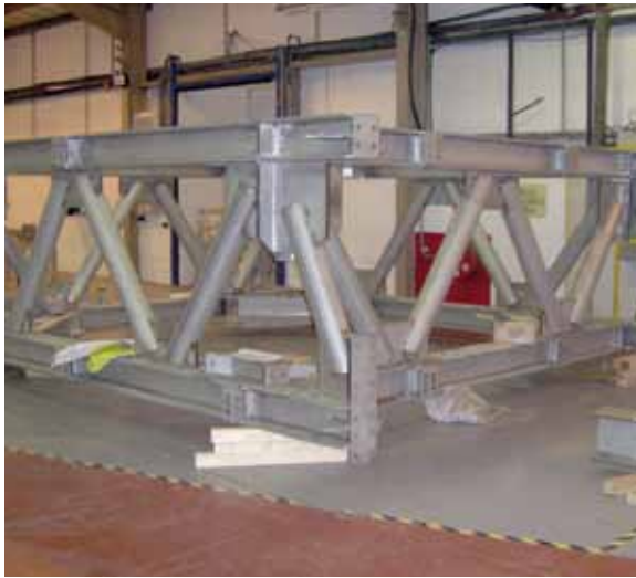
Stainless Steel – Trial Assembly and Pipe Support manufacture at Queensway.
